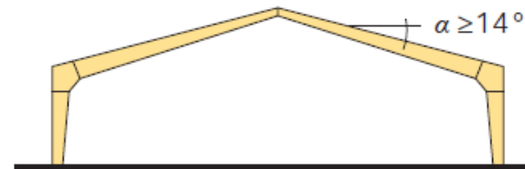
Three-hinged portal frame with finger-jointed haunches
