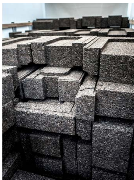
The expanded cork blocks were prefabricated to interlock in plan and section.
