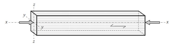
Fig. 1. Element subjected to axial compression stress
